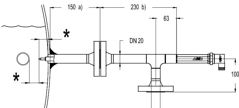
**Vertical installation on a boiler standpipe with a probe flange**
