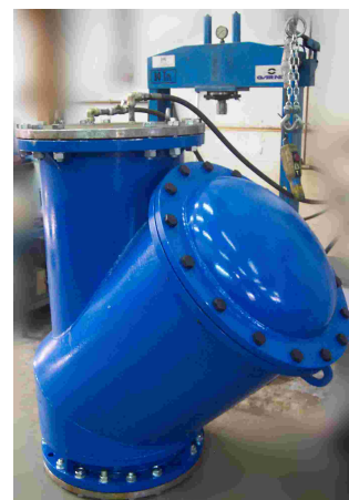
ND500 PRESSURE TEST
