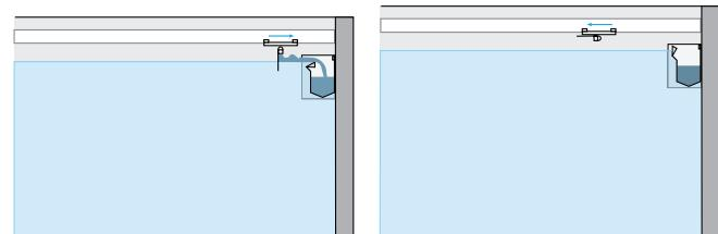
*Only the scraper blade comes into contact with the water surface. When it reaches the end of its travel and has deposited the sludge, the blade is angled up again for the return movement. Several scraper blades can be used in the same tank.*
