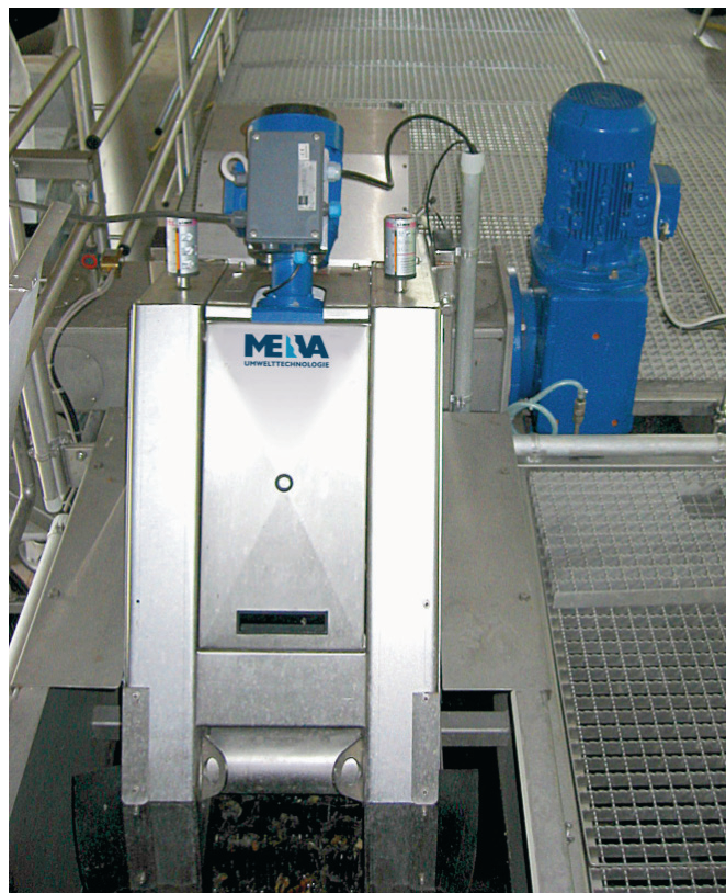
All components in the combi unit are made of stainless steel
