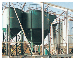
Installation of a treatment plant consisting of a special plate separator and DynaSand filters
