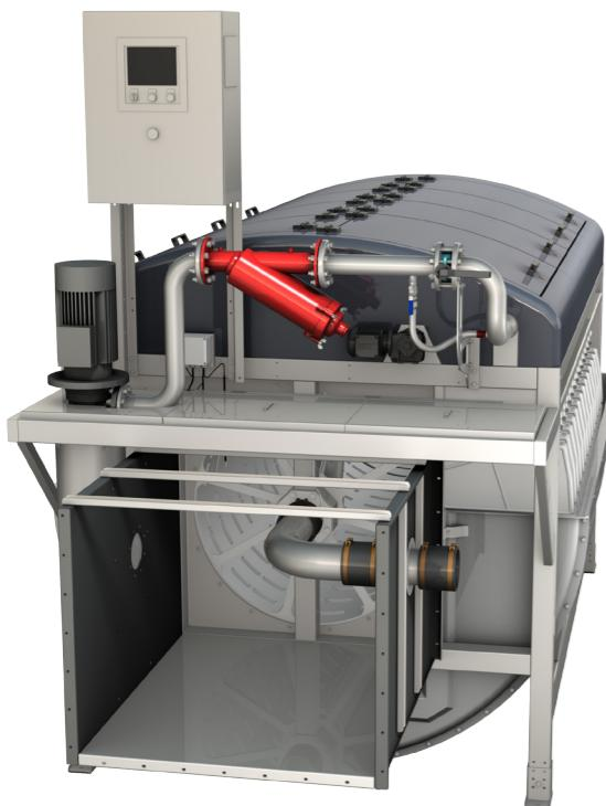
The filter is equipped with an inlet channel connected to the raw water inlet when installed in a concrete tank. The water flows by gravity into the center drum, into the disc cassettes and through the filter cloth.
