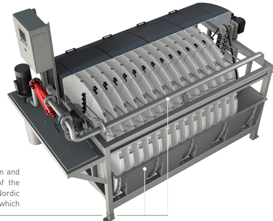
The moving spray bar backwash system and the integrated level tank are some of the specific design details that make the Nordic Water DynaDisc a reliable filtration unit which requires a minimum of maintenance.
