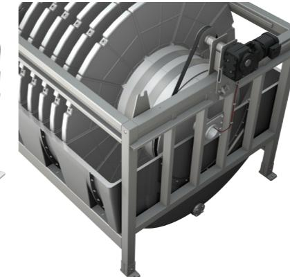
The rotation of the disc filter is driven by a helical-bevel gear drive via a non corrosive synchronous carbon fibre reinforced cog belt.
