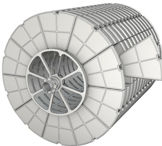
The filter cassettes are easily replaced in a minimum of down-time. Each disc consists of 8 or 10 filter cassettes. The cassettes are easily removed by loosening a nut. The new cassette is then installed by sliding the cassette over the rod and tightening the nut again.
