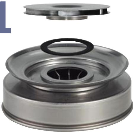
Loss of efficiency has been reduced to an absolute minimum in the impeller stack of the Grundfos CR pumps. This has been achieved for instance by applying a floating seal ring as a perfect seal between the individual chambers.
