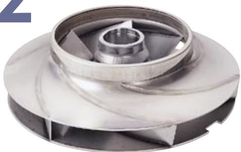
An enhanced impeller/chamber design ensures a more streamlined flow. Tiny margins determine the success of the final result, so Grundfos developed a highly specialised laser-welding technology in order to achieve the highest efficiency on the market for any multistage centrifugal pump
