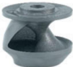
The Grundfos channel impeller pumps provide high efficiency and excellent non-clogging capabilities. The channel impeller of the SE1 range has a free passage of 50 mm. Channel impeller pumps are ideal for heavy-duty operation and for pumping large quantities.
