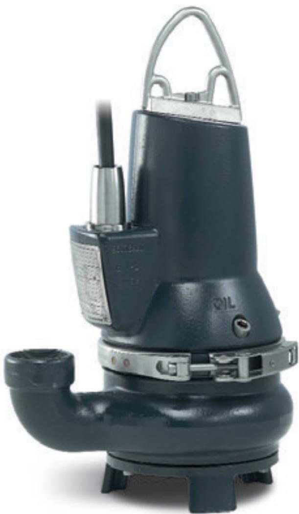
The EF pumps are designed for free-standing installation. The pumps are fitted with an integrated three-leg stand that keeps the suction inlet well clear of the pit bottom. The EF pumps are capable of handling solids of up to 30 mm size.
