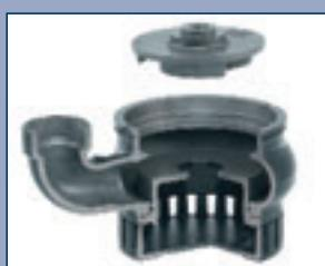
The DP range is fitted with a semi-open multi-vane impeller capable of handling solids up to 10 mm size. The heavy-duty suction strainer is easy to dismantle for cleaning.
