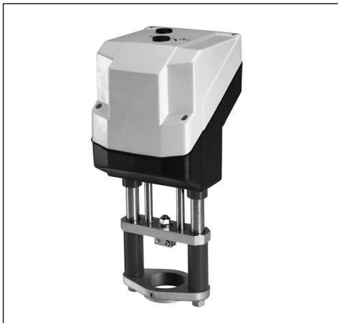
The actuators AMV 85 and AMV 86 are used with VFS 2 valves from DN 65 up to DN 100 diameter or with VF 2 and VF 3 DN 125 and DN 150 diameter. The actuator automatically adapts its stroke to valve end positions which reduces commissioning time.
