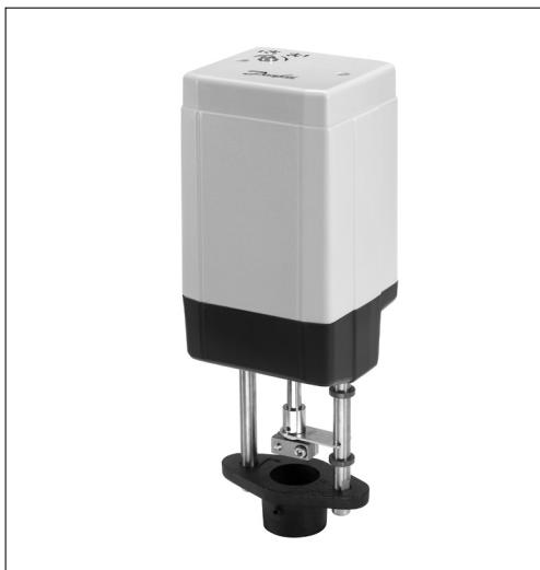
The actuators AMV 55 and AMV 56 are used with VL 2, VL 3 and VFS 2 valves from DN 65 up to DN 100 diameter and VF 2, VF 3 valves from DN 65 up to DN 150 diameter.
